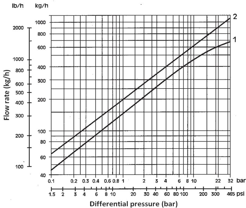
Curve 1: discharge 10 °C below the saturated curve
